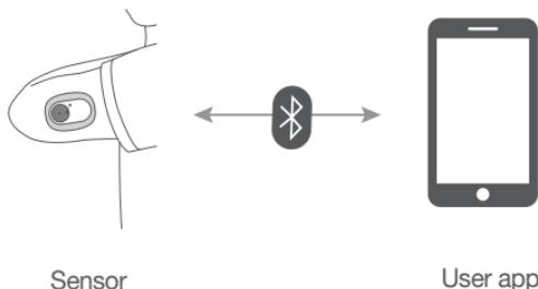
The user attaches the sensor to their body by pressing the Release button of the applicator. The sensor attached to the back of your upper arm measures glucose levels in interstitial fluid and sends the measurements to a smart device.
