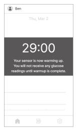
Once the sensor warmup is completed, the glucose reading will be displayed and will change from gray to blue. If needed, you can tap the blue to enter a calibration value.
