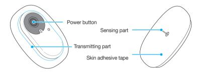
The table below shows the names and functions of the sensor's various parts.
