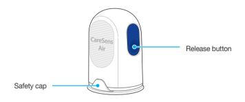
The following names are used for the parts of the applicator:
