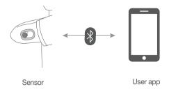
The user attaches the sensor to their body by pressing the Release button of the applicator. The sensor attached to the back of your upper arm measures glucose levels in interstitial fluid and sends the measurements to a smart device.
